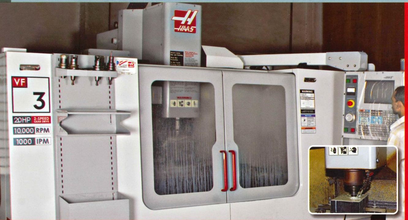
HAAS make CNC Vertical Milling Machine Centre with 20 Station ATC & pneumatic clamping, Fanuc Control for the machining of any type of Die, high surface finish on Dies.
